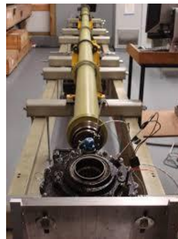
Figure 4. IGB on no-load test stand (Top) and close-up of the IGB used for the testing (bottom)
