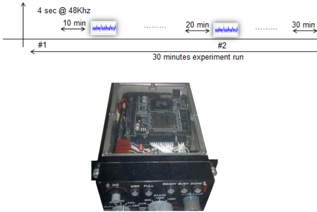
Figure 5. Vibration data acquisition on the no-load stand (Top) and the MSPU (bottom)
