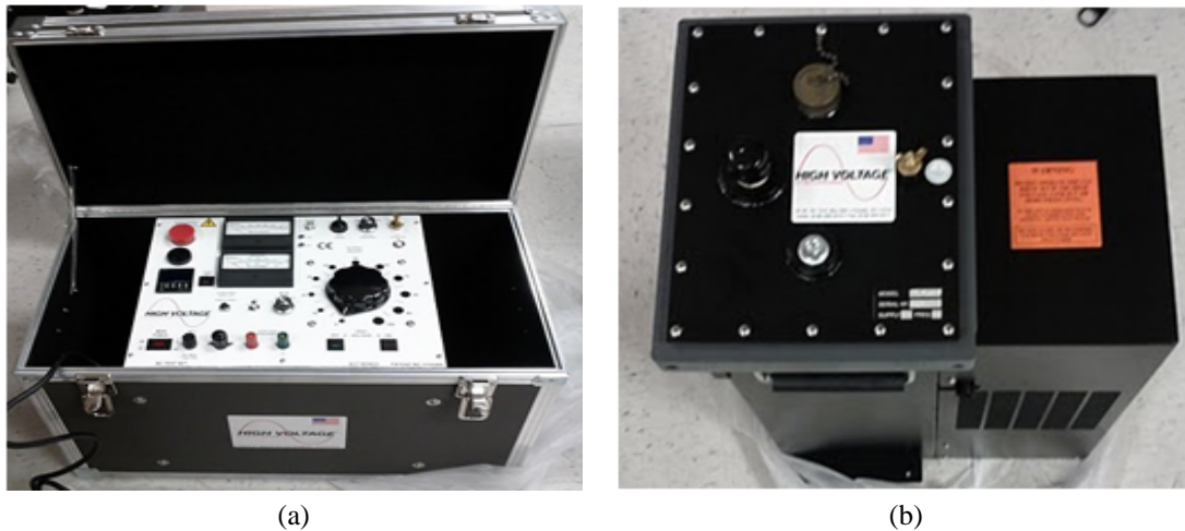
Figure 16: Very low frequency source (VLF) operates at frequencies from 0.02-0.1Hz, simulating line frequency of 50 or 60 Hz, for high voltage tests up to 50kV with (a) controller, timer, and measurement unit and (b) high voltage tank capacitor
