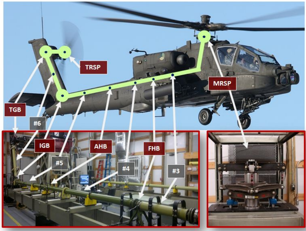
Figure 1.4: TRDT/MRSP in actual AH-64D (Top) and TRDT/MRSP test stands at USC (Bottom)
