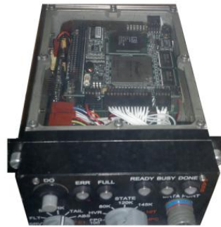
Figure 1.5: Example of MSPU used on AH-64 (Intelligent Automation Corporation: VMEP Crew Member Information Guide)
