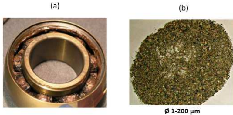
Figure 5.3 Faulted AHB: (a) assembled bearing, (b) zoom-in view of the coarse grit contamination
